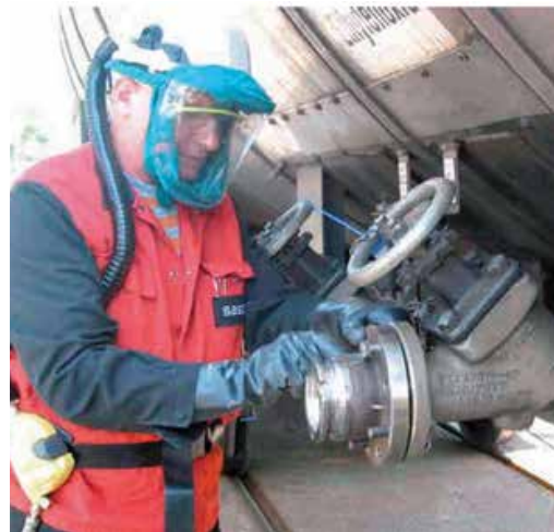
Fig. 10 Fully protected operator checking for a spill
