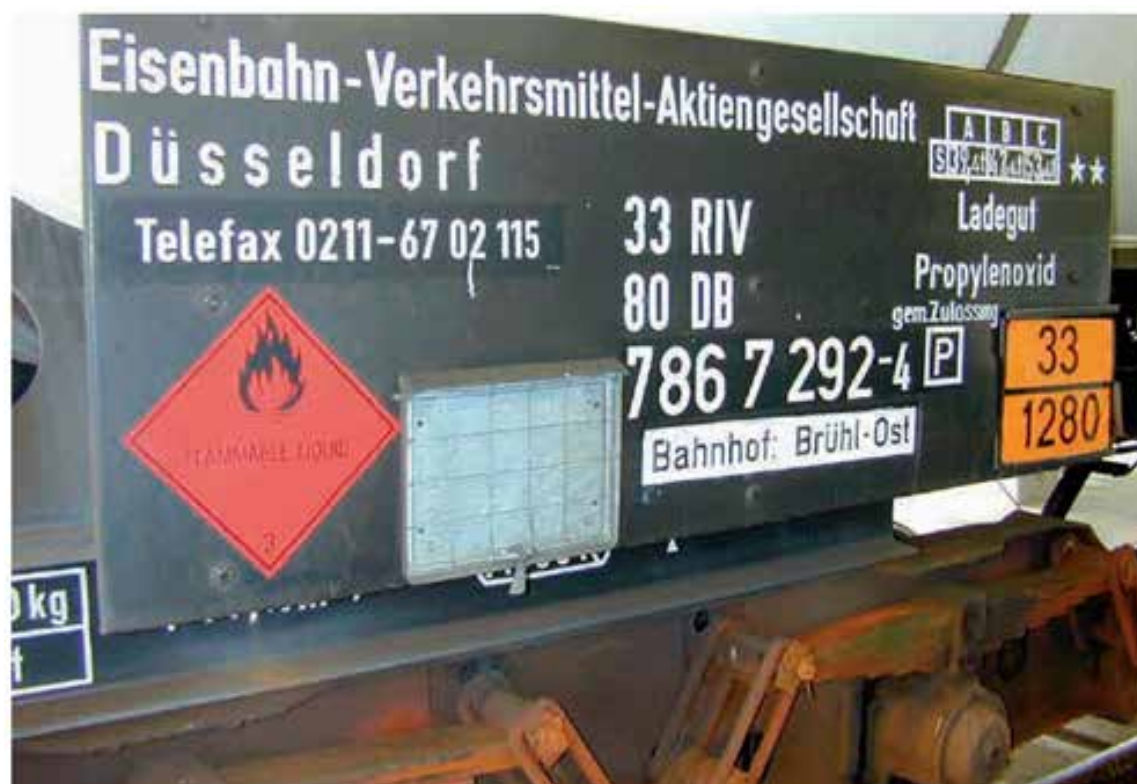
Fig. 1 Legend table of a Propylene Oxide rail car
