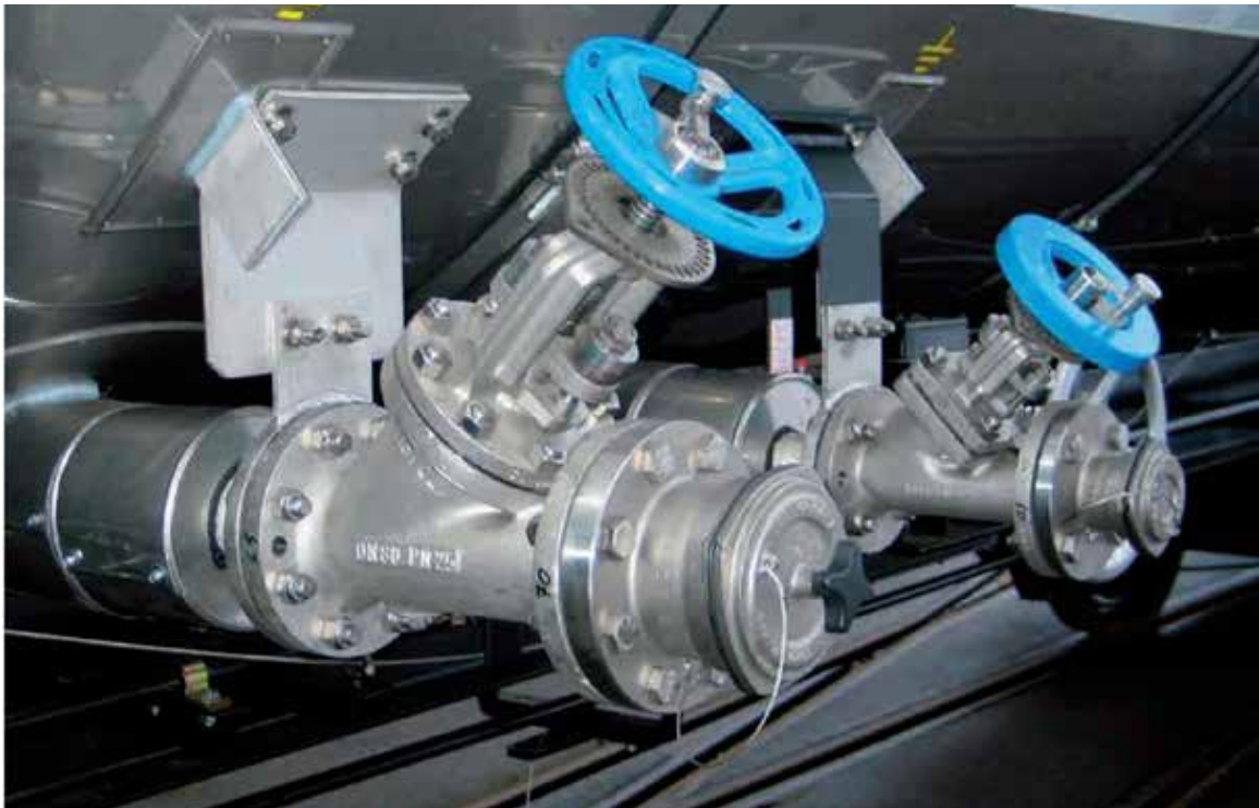
Fig. 2 Dry Disconnect Coupling connection
