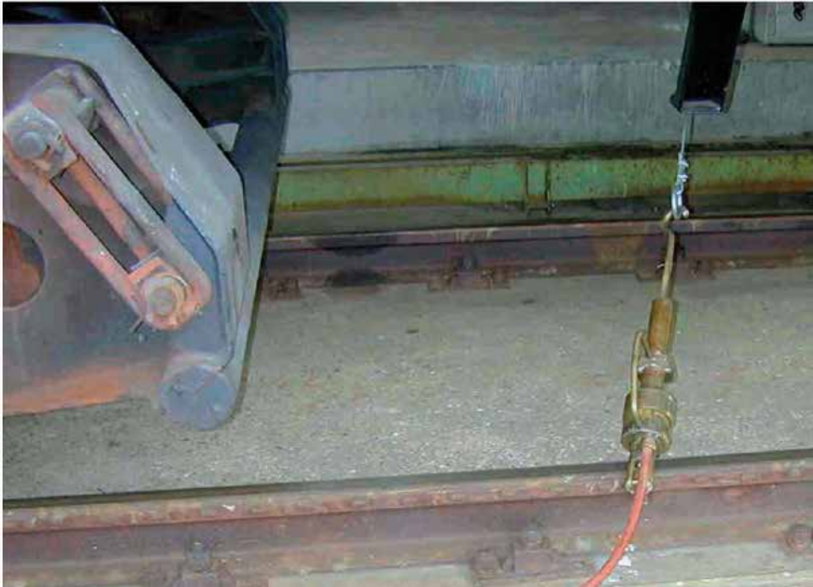
Fig. 9 Rail hook combined with a remote control, which closes the bottom valve if activated. This example shows only the set up for liquefied gas railcars.
