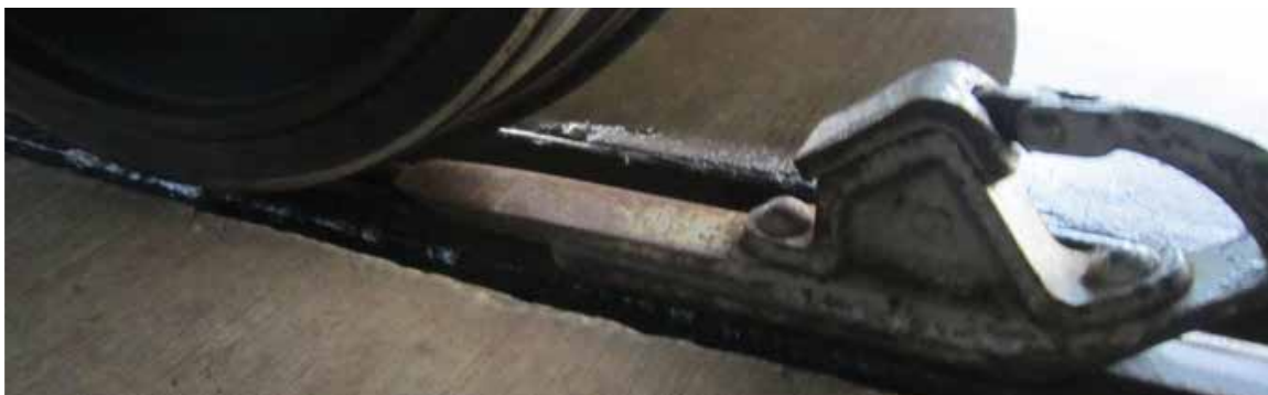
Fig. 8 Blockade to fix a rail car
